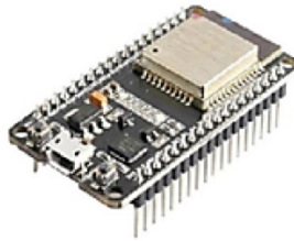
Fig. 4. ESP32 microcontroller used for sensor data aggregation and wireless transmission [20]
