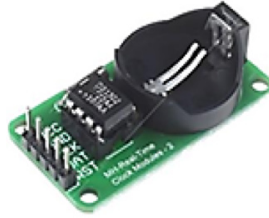
Fig. 3. DS1302 real-time clock module for synchronized data acquisition [19]
